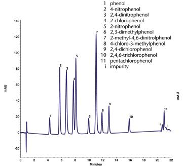
Column: Eurospher II 100-3 C18 P 100 x 3 mm Mobile phase: A: water (+ 0.1% formic acid)
