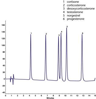
Column: Eurospher II 100-3 C18 P 100 x 3 mm Mobile phase: A: water (+ 0.1% formic acid)
